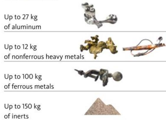
Metals and inerts for reuse recovered from bottom ash.
