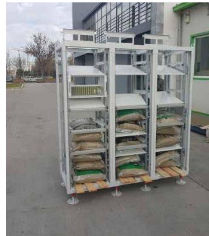
LIFTING TEST 210Kg's for each column
