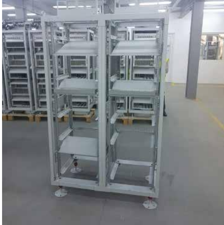
LIFTING TEST 210Kg's for each column
